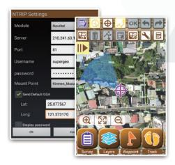
▲ NTRIP solution allows you to reach sub-meter accuracy
