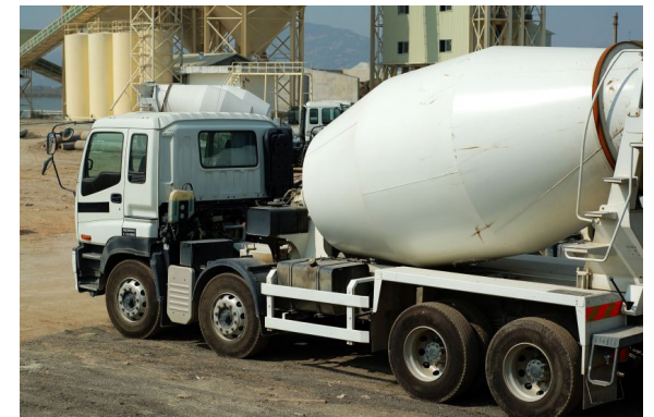
Ready Mixed Concrete (RMC) is the indispensable raw material for constructions, and would be delivered to the construction sites by ready mixed concrete trucks.
