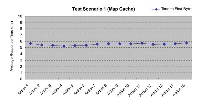
In the test, we record the related data of the two servers handling 30 users' requests at a time, and make a chart to show the results. From the chart above we learn that the website supporting cache function spends almost the same time obtaining each piece of map when the website is manipulated by multiple users for a long time. Furthermore, after 30-minute continuous access, the website can still offer the multiple users the high stability web
